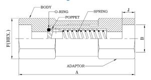
It is used to prevent backflow. \*Backflow simply means the flow that has reversed itself within the pipe and begins to flow backwards. It is used for unidirectional flow. (Special requirements available on request)
