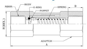
It is used to prevent backflow. \*Backflow simply means the flow that has reversed itself within the pipe and begins to flow backwards. It is used for unidirectional flow. (Special requirements available on request)
