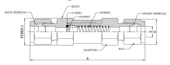
It is used to prevent backflow. \*Backflow simply means the flow that has reversed itself within the pipe and begins to flow backwards. It is used for unidirectional flow. (Special requirements available on request)
